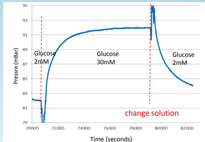
**Fig.3: Dose response curve for the sensor signal at different glucose concentrations using dextrane 40kDa**
