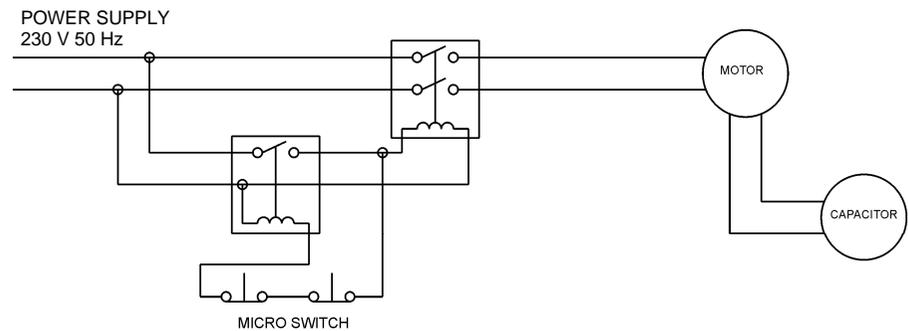
FIG. n°5 - Electrical layout
