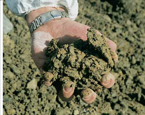
Before: sticky raw material with adhering fine content and agglomerates
