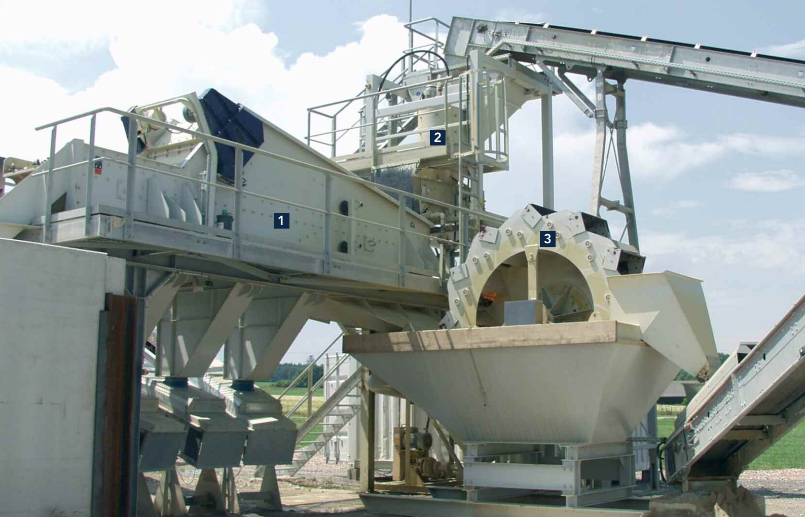
System technology: 1 Classifying screen – 2 HYDRO-CLEAN® – 3 Scoop wheel
