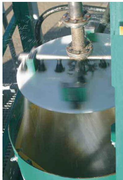
Washing rotor with rotating high-pressure water jets
