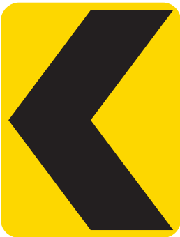
CHEVRON ALIGNMENT MARKER D4-6A 600 x 750mm D4-6B 750 x 900mm D4-6C 900 x 1125mm
