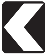
UNI DIRECTIONAL HAZARD MARKER D4-1-2A 450x450mm D4-1-2B 600x600mm
