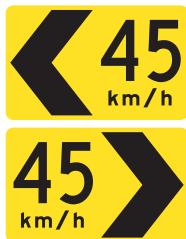
CHEVRON WITH SPEED D4-V110A 1200 x 750mm D4-V110B 1500 x 900mm D4-V110C 1800 x 1125mm
