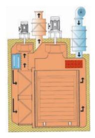
HEPA filters on the recirculation wall have a gasketless vacuum sealing system, which eliminate particle shedding and filter gasket maintenance.
