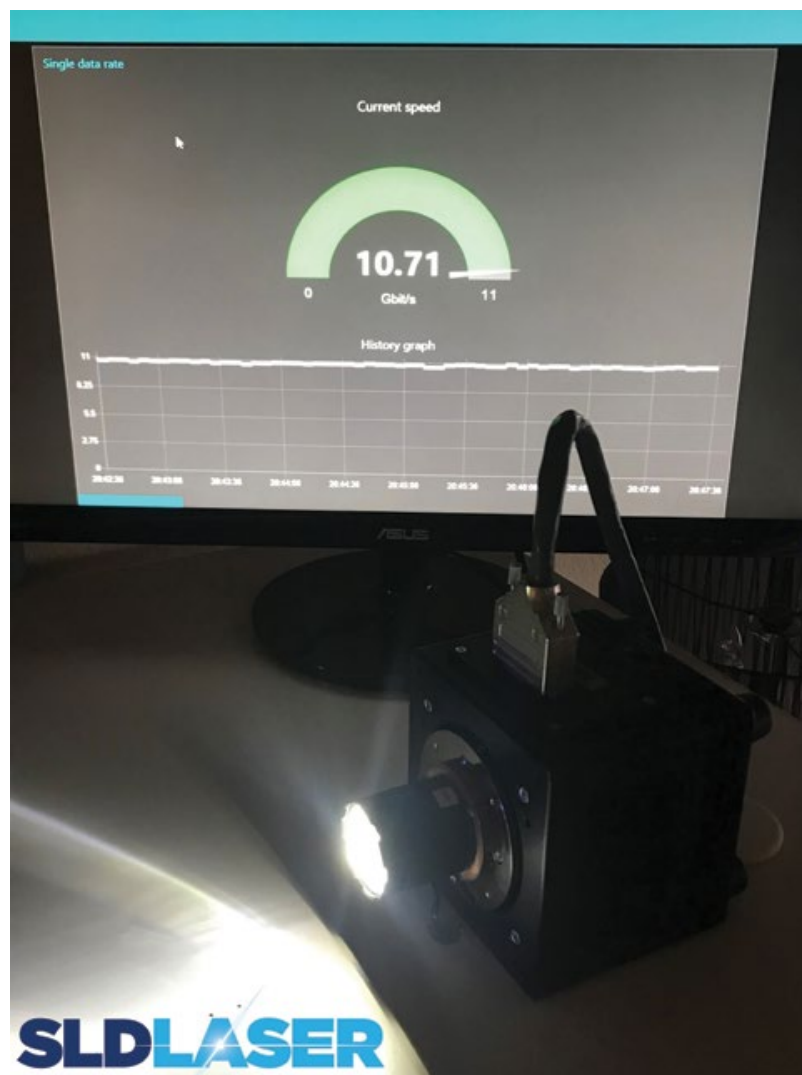
LaserLiFi can now deliver >10Gbit/sec at 5 meter range from a 500 lumen spotlight. Image courtesy of SLD Laser
