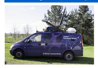
Single path trucks with single ca mera input. Used regularly to provide small-scal e add-ons to a host OB feed for sports, live events, news, corporate clients. The vehicles house a Nimbra 640 unit as well as retaining uplink capability (up to 18MHz). UPS, generator power back-up.
