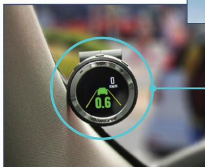
The EyeWatch<sup>™</sup> display for visual alerts, mounted in vehicle's cabin
