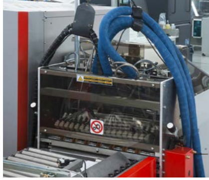
Hot melt application by extruder nozzles
