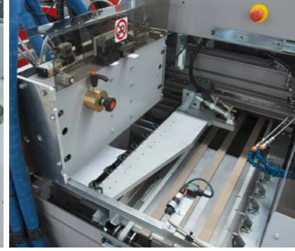
Sheet transfer after glue application
