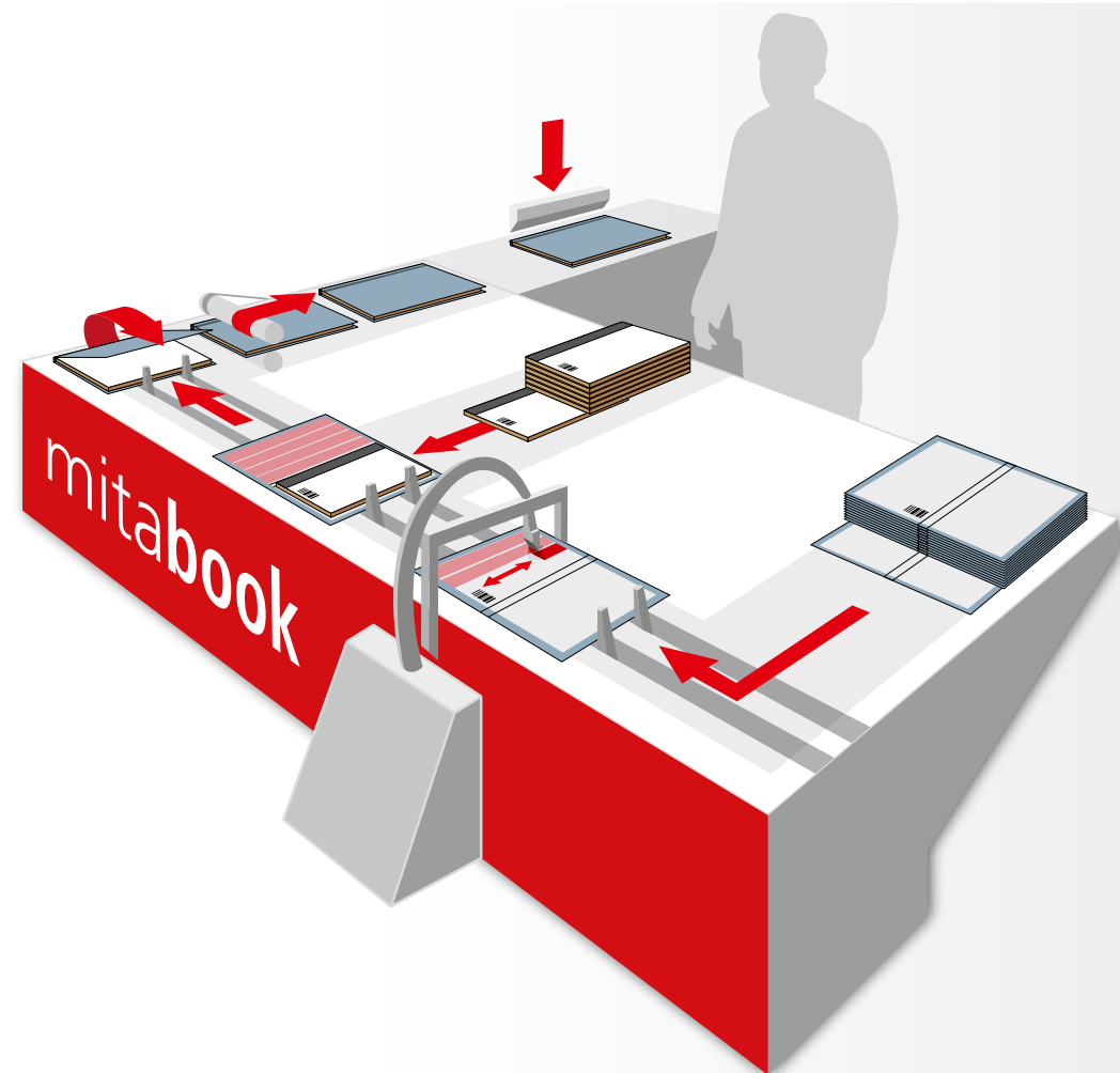
Closing and initial pressing of the cased-in book prior to joint-forming
