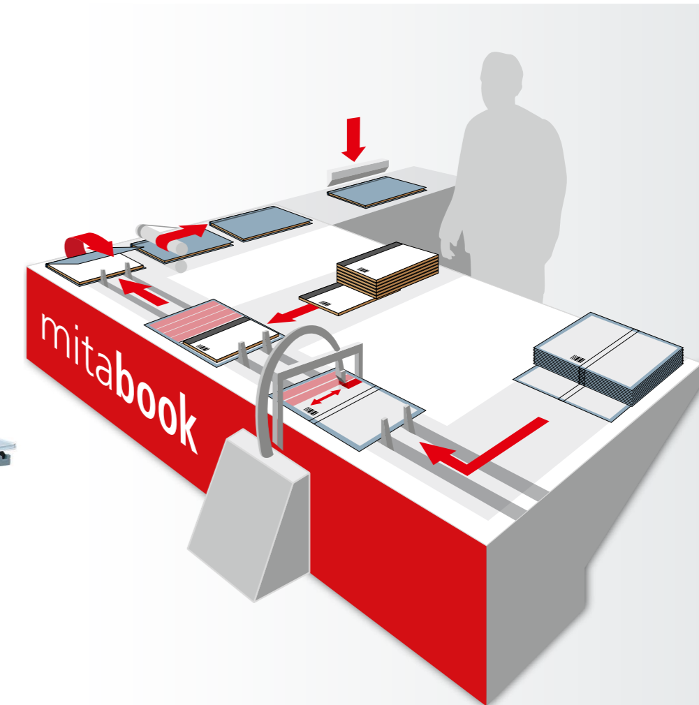
Automatic production mode with blocks of different thicknesses and spine in-lays with corresponding widths (optional)
