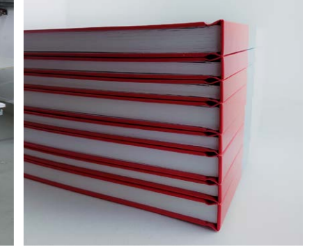
Automatic production mode with blocks of different thicknesses and spine in-lays with corresponding widths (optional)
