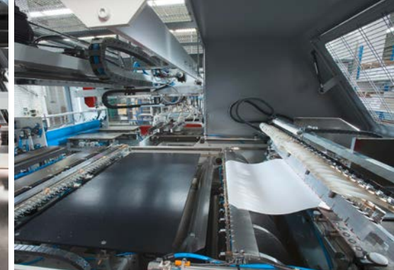
Cover transport over gluing roller to vacuum table
