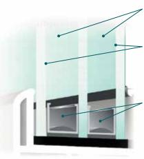
**Argon** is an insulating gas between the glass panes that acts as a thermal barrier on energy loss, counteracting heat and cold conduction. Argon gas also helps reduce noise infiltration for a quieter indoor ambiance.
