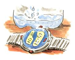
Pour some water into the top and time how much water drips through in 1 minute, 2 minutes, 3 minutes and so on.
