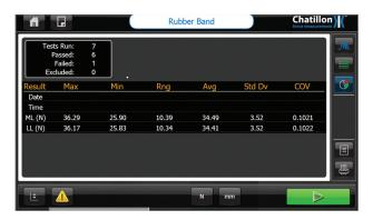
Choose statistic results to display for complete batch tests.
