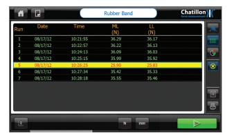
View batch test results. Exclude non-compliant test runs.
