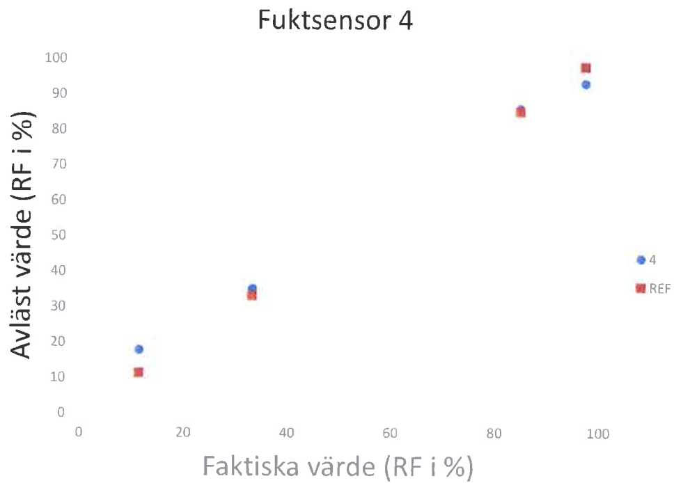
Figure 13. RH Sensor “-4”. Results from the post experiment saturated salt solution check. The squares “REF” show the true values (x -axis), whereas the circles show the instrument read values (y axis).
