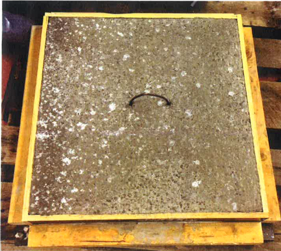
Figure 2. HPC 100 concrete slab. The dimensions of the surface area is 0.5 m x 0.5 m .This slab is 0.1 m thick. Note the rebar in the middle, this was cast in order to aid the weighing.
