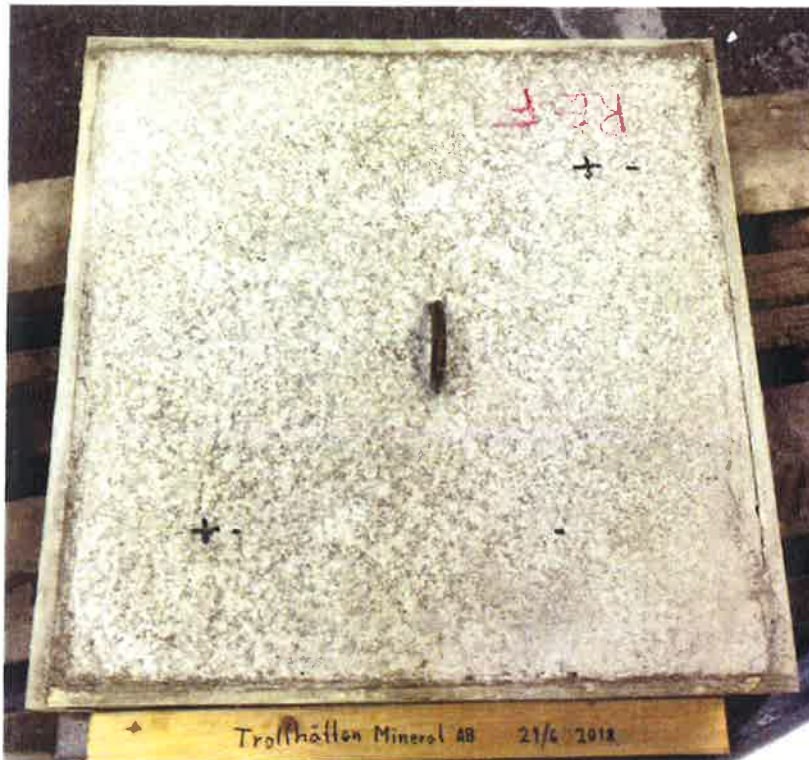
Figure 1. Reference concrete "REF". The "+" signs mark the positions where the measurement holes were to be drilled. The dimension of the concrete is 0.5 m x 0.5 m. The thickness of this slab is 0.2 m.
