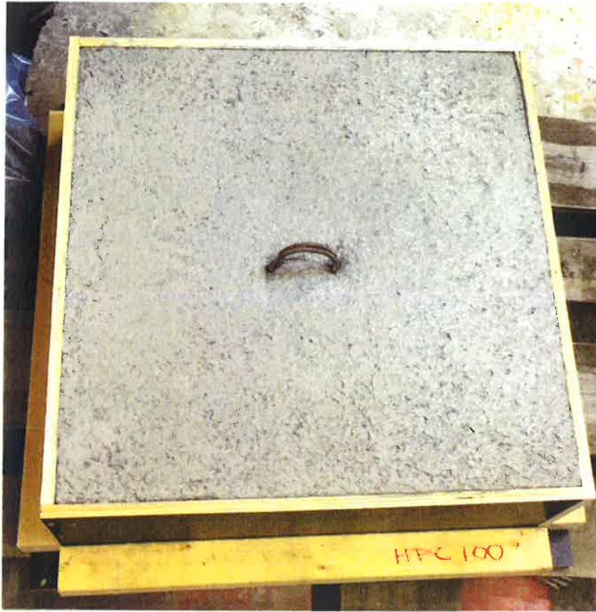
Figure 3. HPC 100 concrete slab. The dimensions of the surface area is 0.5 m x 0.5 m. This slab is 0.2 m thick.
