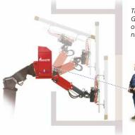
The special construction of the Gerenuk® 500 allow e.g. fitting of windows and doors on balconies from the outside.
