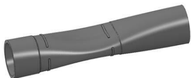
Fig. 2: Collapsed pipe from side
