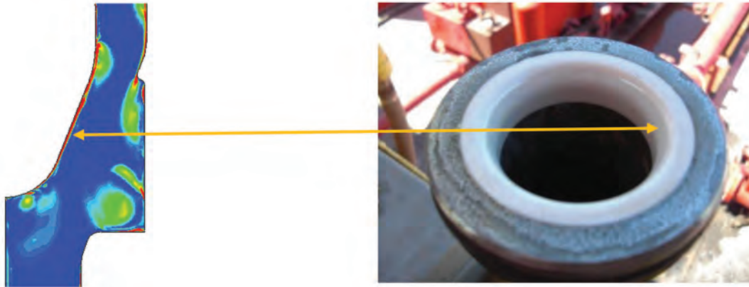
Fig. 3: Erosion effects after 10 hours on optimized design of mud valves (top and bottom)
