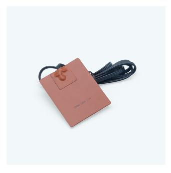
Silicone Heating Pads are ideal for oil pans, engine blocks, hydraulic reservoirs, diesel fuel tanks and other fluid reservoirs. Constructed from a durable silicone/fiberglass material, these etched foil heating pads feature an easy peel-and-stick application. Silicone heating pads are for use on metal surfaces only; do not use on batteries.
