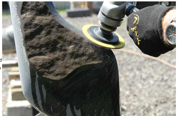
PMG PHOTO: SAM STITES - The polishing process to gain the funhouse mirror effect Haslett is going for takes seven steps at varying degrees of diamond grit.
