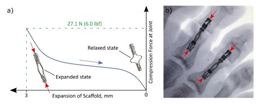
Figure 1: a) Schematic of compression force at the joint versus expansion of scaffold. b) X-ray of two implanted SuperScaffold<sup>TM</sup> devices.
