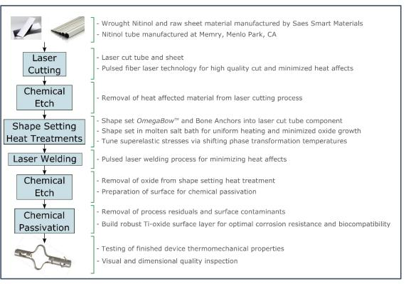
Figure 3: Memry's manufacturing process flow.
