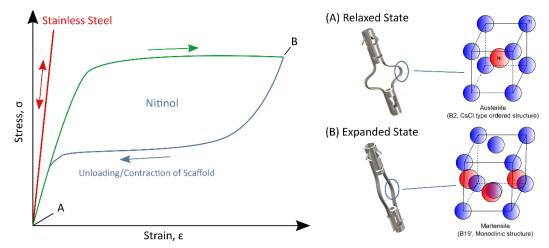
Figure 2: Typical Nitinol cyclic superelastic stress-strain curve & relation to Nitinol crystal structure and device state. A) Device in unstrained/relaxed state with the Nitinol material in the Austenite phase & B) Device constrained in an elongated/expanded state with Nitinol material in the Martensite phase.
