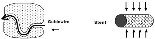
Kink and crush resistance are directly proportional to superelasticity therefore one must ensure that the application or design fit well within the superelastic temperature range. This range is highly sensitive to heat treatment conditions. Both superelastic range and fatigue properties beneficiate from a high UTS to loading plateau stress ratio. Once again and because of temperature dependencies, design and manufacturing must focus on the device operating conditions.
