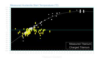
Figure 1: A plot of measured austenite start (As) temperature versus charged (o) and measured (•) titanium contents (Courtesy of Special Metals Corporation).
