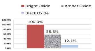
Figure 5: Fractures by Oxide Level, High and Low Strain, Single Wire Only, Ø0.008" Wire.
