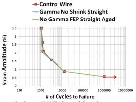
Figure 9: Strain-N NiTi Control Samples.
