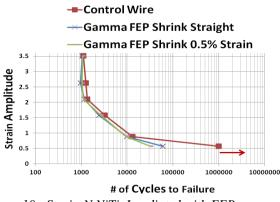
Figure 10: Strain-N NiTi Irradiated with FEP.
