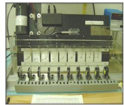
Figure 8: Rotating Beam Test Apparatus.
