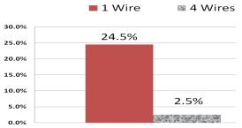
Figure 4: Fractures by Number of Wires, High and Low Strain, 0.008" Wire, All Oxide Levels.
