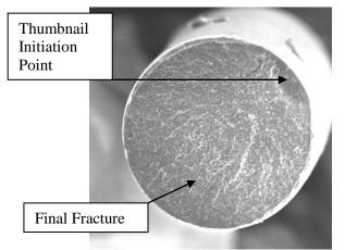
Figure 7: SEM Image of Post Gamma SCC.
