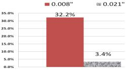
Figure 3: Fractures by Wire Diameter, High and Low Strain, Single Wire Only, All Oxide Levels.
