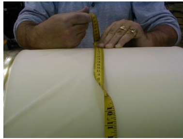
Figure 3: Incorrect Measurement because tape is twisted.
