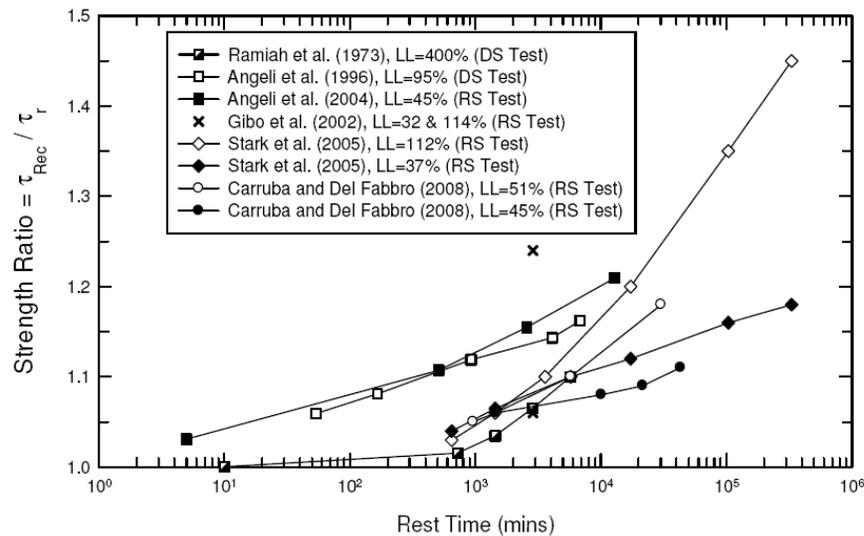
**Figure 1. Summary of published strength recovery test results for effective normal stress of 100 kPa or less**
