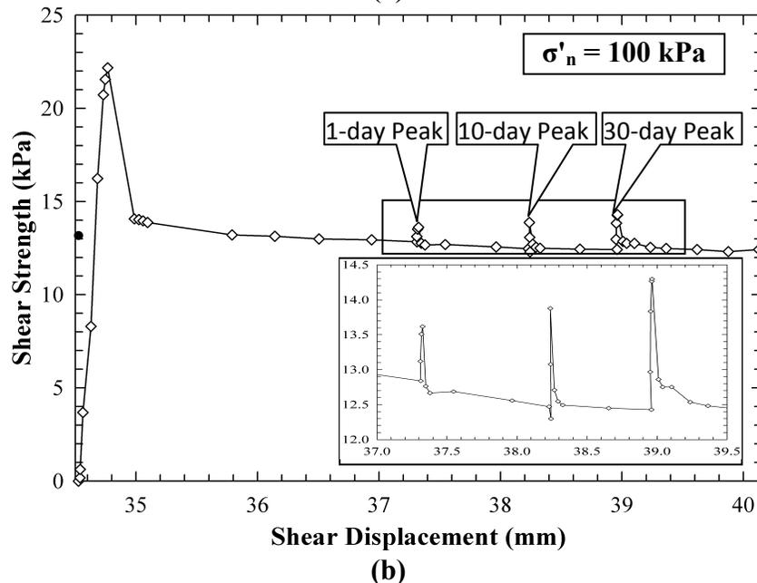
**Figure 3. (a) Complete test results for direct shear strength recovery test at an effective normal stress of 100 kPa and (b) third cycle during which specimen subjected to various rest periods.**
