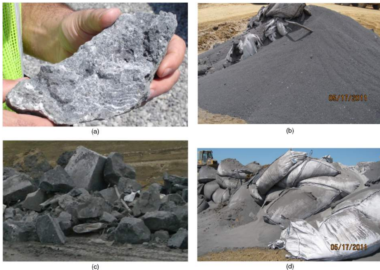
Fig. 1. Types of aluminum production waste: (a) white dross; (b) black dross (from Site 2); (c) salt cake; (d) baghouse dust (from Site 2)
