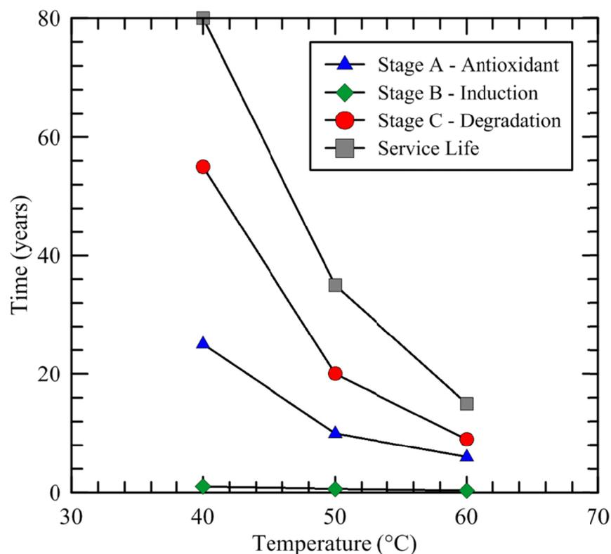
**Figure 2. Duration of degradation Stages A-C and total service life based on 50% reduction in tensile strength at break (data from Rowe 2005).**
