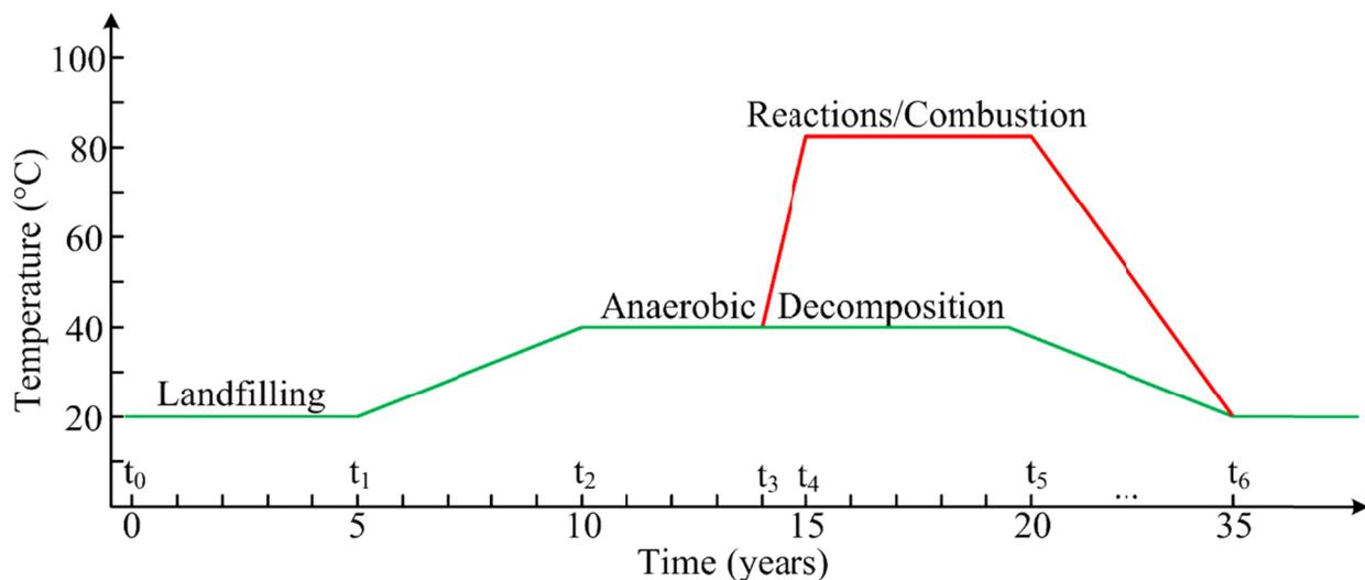
**Figure 3. Idealized time-temperature history in a landfill under elevated temperatures.**
