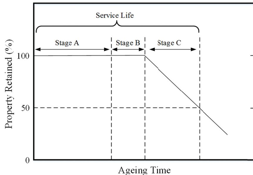
**Figure 1. Conceptual diagram of service life and the three stages of degradation: Stage A antioxidant depletion; Stage B induction time; and Stage C polymer degradation and reduced physical and/or mechanical property (modified from Hsuan and Koerner 1998).**
