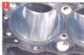
With MTC, the cylinder walls are clean from any build-up, and look highly polished
