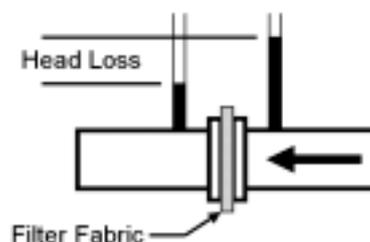
Figure 2. Experimental setup of Catchpit
