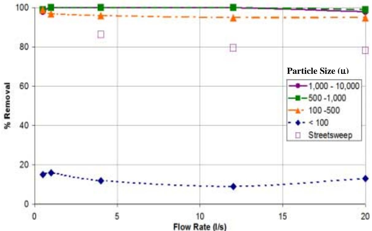
Figure 4 above shows the results in the standard catchpit without a CFS installed. Sediments larger than 500 $\mu$  were completely removed for flows up to 20 l/s. The removal of 100-500 $\mu$  particles decreases from 75% to 47% by increasing the flow from 0.5 l/s to 20 l/s, and only 18% of particles smaller than 100 $\mu$  are trapped by the catchpit. Approximately 58% of the sediment collected from street sweepings were removed at 4 l/s.
