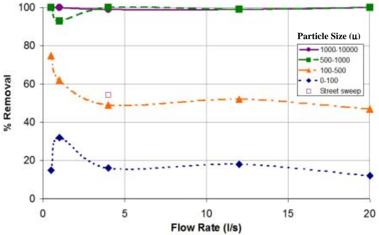
Figure 5 - Sediment Removal by the Catchpit Containing an Enviropod CFS with a 200 µm mesh
