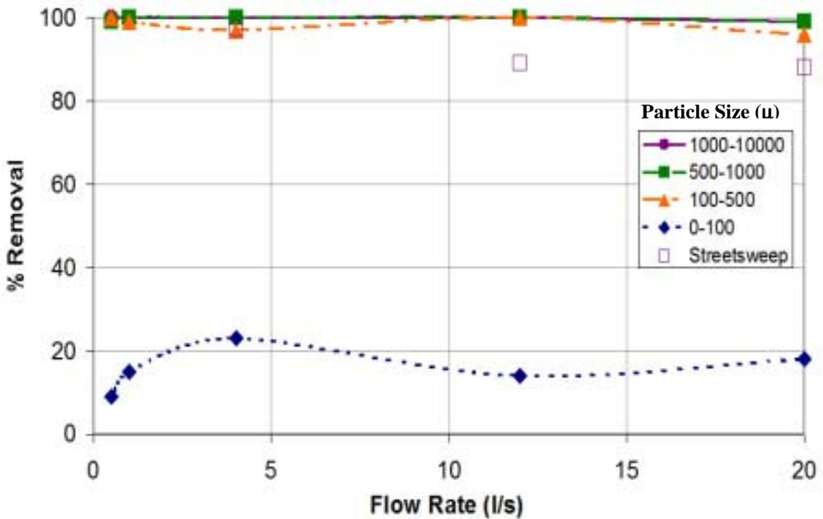
Figure 6 - Sediment Removal by the Catchpit Containing a Flogard CFS with a 400 µm mesh
