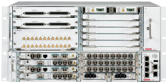
Figure 1. 6200 Base + Expansion Chassis Configuration
