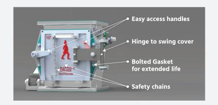
The unique hinged cover design integrates double hinge technology with our already popular easy access camlock cover. This innovation is an option for both new or existing valves in the field and can be easily retrofit by Plattco service technicians or maintenance personnel.
