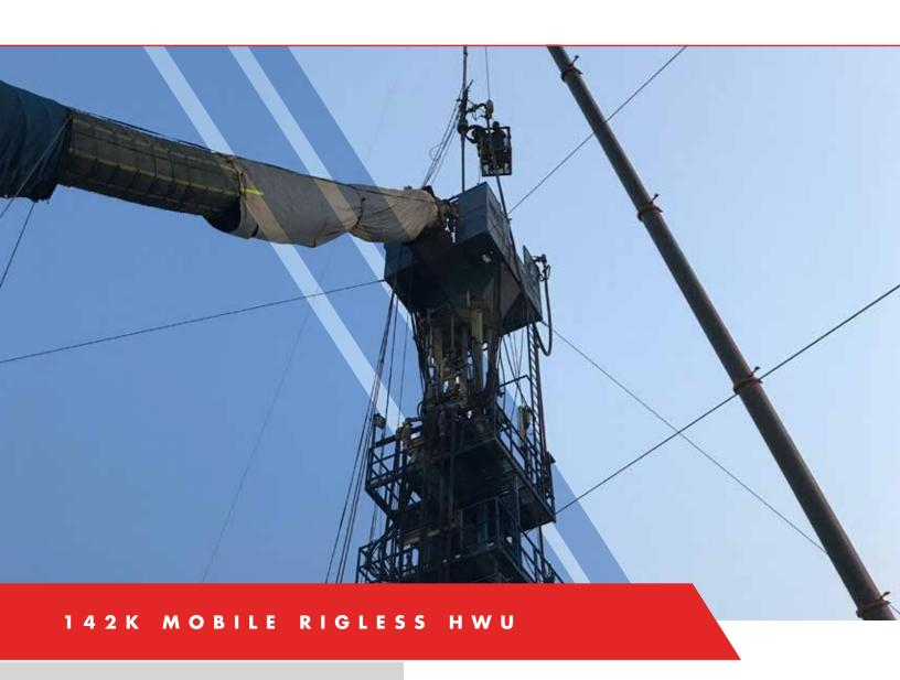
A reliable, fully mobile unit that comes complete with an optional 10K primary BOP, 10K pump and internal BOP guides for high pressure situations.
